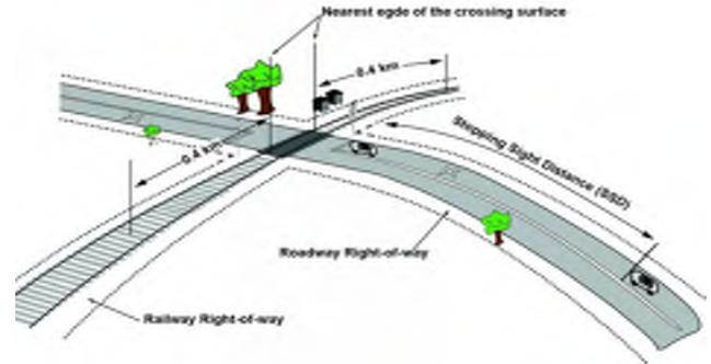
Figure D-1 - prescribed area for whistling cessation as per article 23.1 of the RSA
