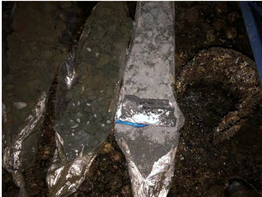
Photograph 4.1: Glacial till core samples.
