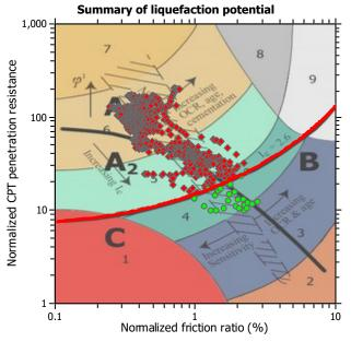
Zone  $A_1$ : Cyclic liquefaction likely depending on size and duration of cyclic loading Zone  $A_2$ : Cyclic liquefaction and strength loss likely depending on loading and ground geometry
