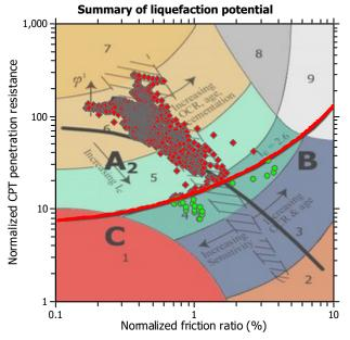
Zone A<sub>1</sub>: Cyclic liquefaction likely depending on size and duration of cyclic loading Zone A2: Cyclic liquefaction and strength loss likely depending on loading and ground
