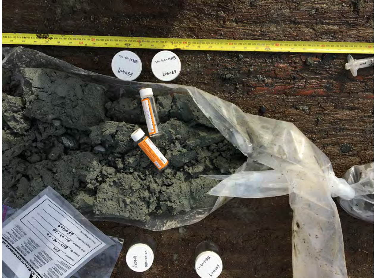
Photograph 2: Retrieved cored sample – sand fill from BH21-04-02 (approximately 1.7 m below mud line).
