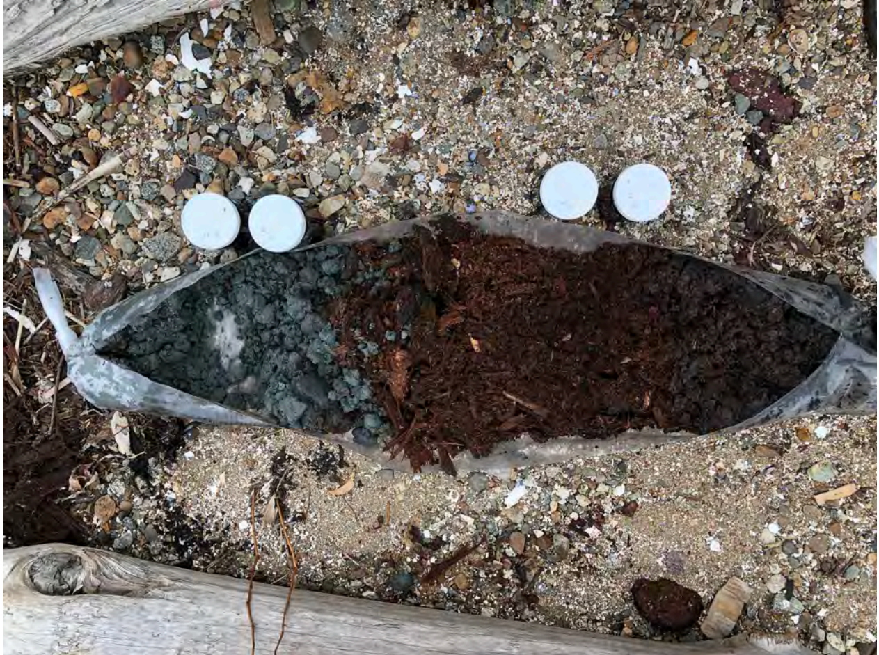
Photograph 2: Sediment sample of lower woodwaste layer and underlying till-like grey sand and silt from BH21-14-05 (approximately 3.7 m bgs)
