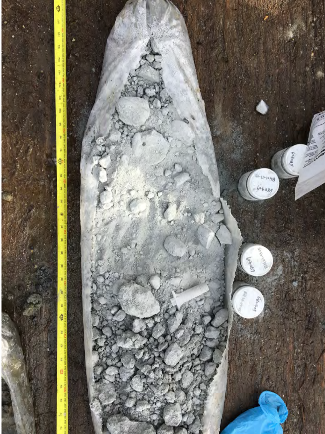
Photograph 3: Retrieved cored sample – till-like sand and gravel from BH21-03-05 (4 m below mud line).
