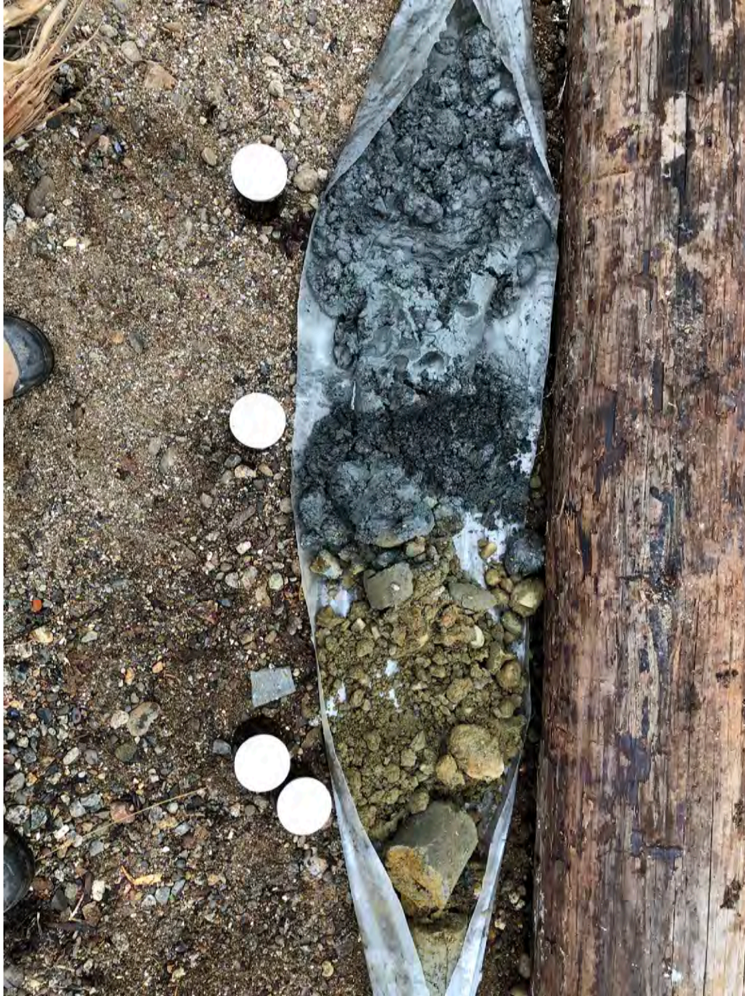
Photograph 3: Sediment sample of grey sand and underlying till-like silt (light brown colour) from BH21-16 (~2 m bgs)
