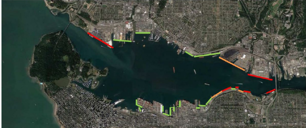
Figure 1: Tidal Current Zones for planning (Red = fast, Orange = moderate, Green = slow) – Ref [2]
