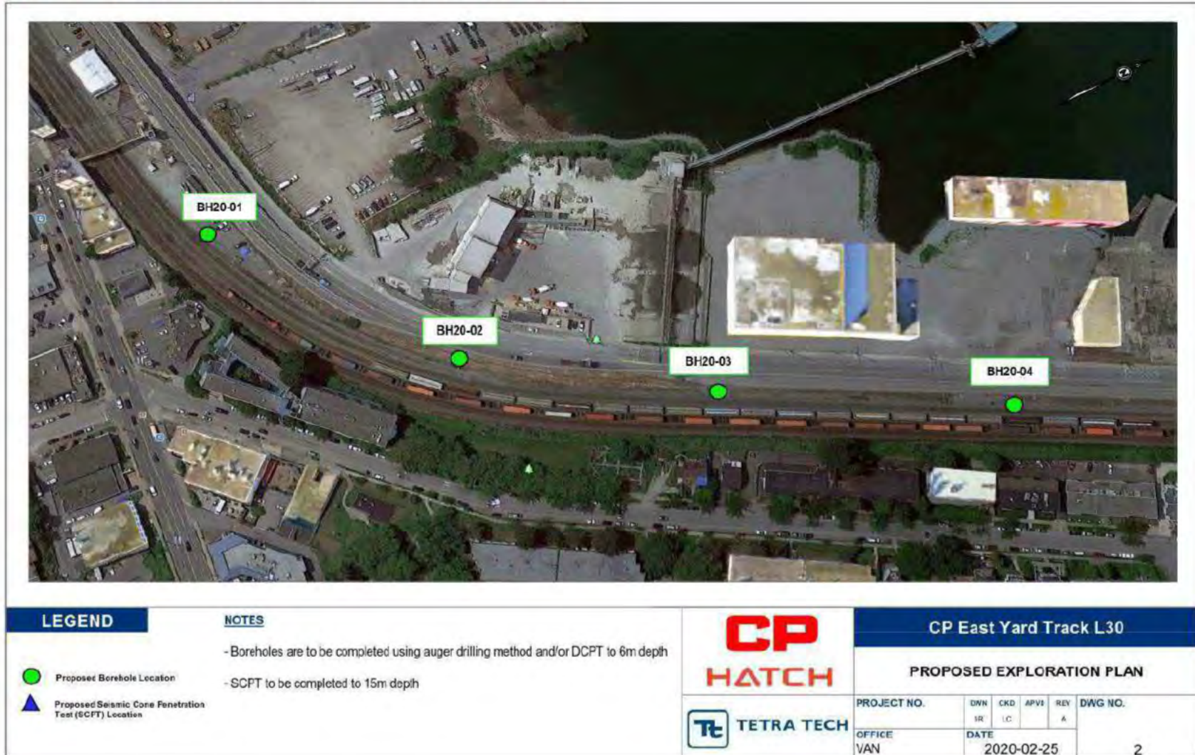
Figure 3: Proposed Borehole Locations – BH20-01 through BH20-04
