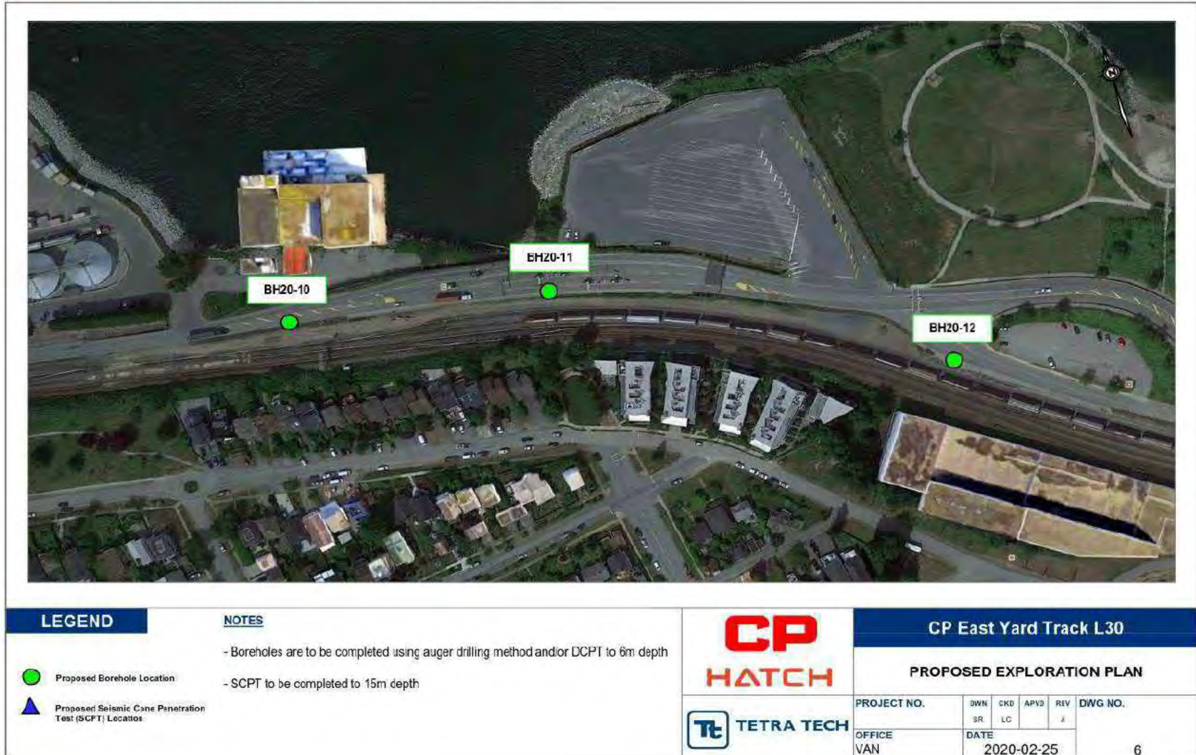
Figure 7: Proposed Borehole Locations – BH20-10 through BH20-12
