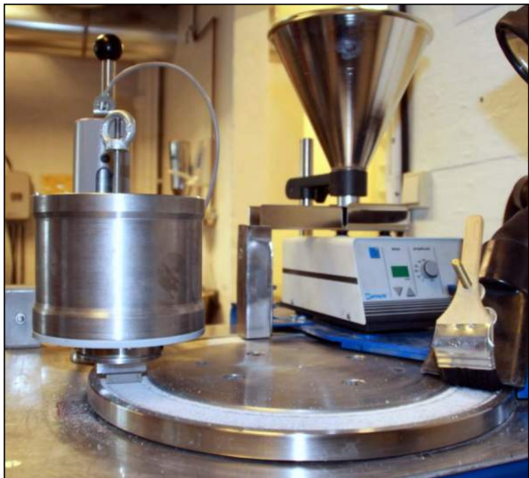
Figure 3. Photos of test equipment used to determine soil abrasivity by the Soil Abrasion Test (SAT™).
