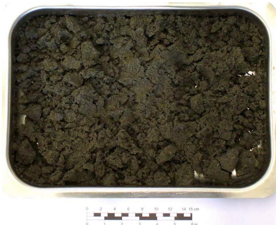
Sample No. 2, "SH16-05, SA#39 105'-106'6". The SAT™ powder was prepared by sieving with steel balls. Of the total sample volume, 100 % was < 1.0 mm after preparation.
