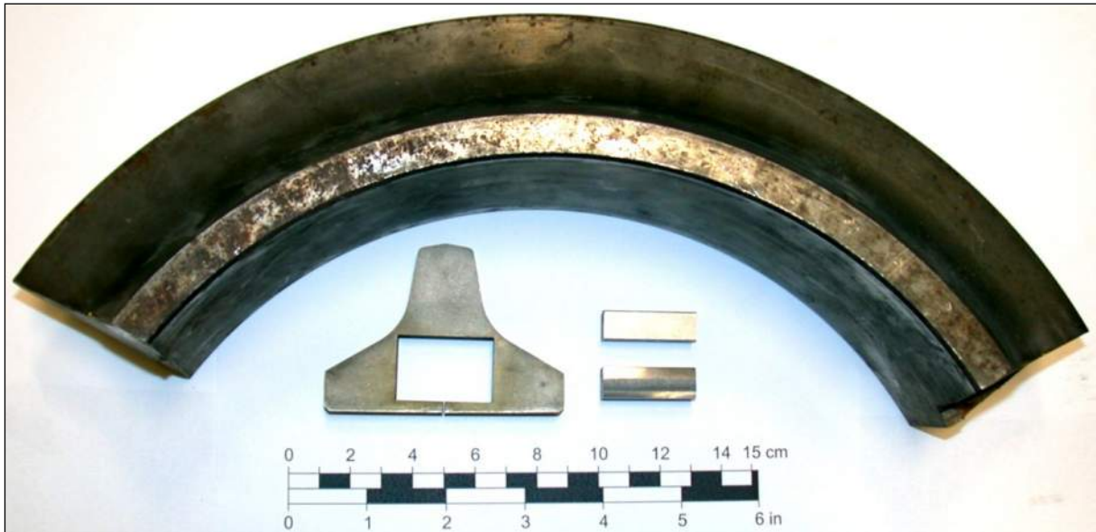
Figure 4. Photo showing a part of a cutter ring, a 10 mm slice taken from the same ring, and two prepared AVS test pieces which are cut out of the center of the slice.
