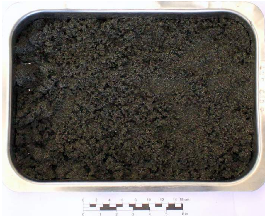
Sample No. 1, "SH16-07, SA#40 105'-106'6". The SAT™ powder was prepared by sieving with steel balls. Of the total sample volume, 100 % was < 1.0 mm after preparation.
