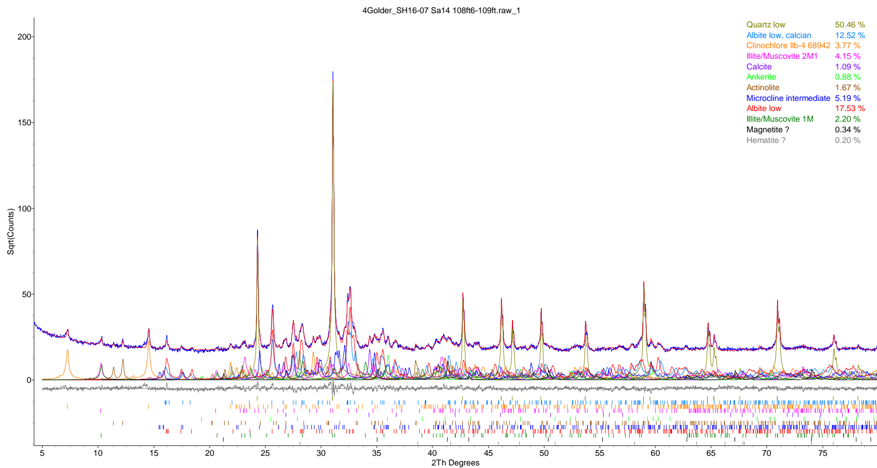
Figure 3. Rietveld refinement plot of sample Golder Associates SH16-01 Sa47 108'3"-109'9" (blue line - observed intensity at each step; red line - calculated pattern; solid grey line below - difference between observed and calculated intensities; vertical bars - positions of all Bragg reflections). Coloured lines are individual diffraction patterns of all phases.
