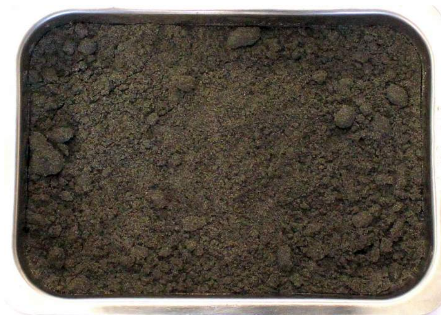
Sample No. 3, "SH16-06, SA#40 106'6"-108'3". The SAT™ powder was prepared by sieving with steel balls. Of the total sample volume, 98 % was < 4.0 mm and 94 % was < 1.0 mm after preparation.
