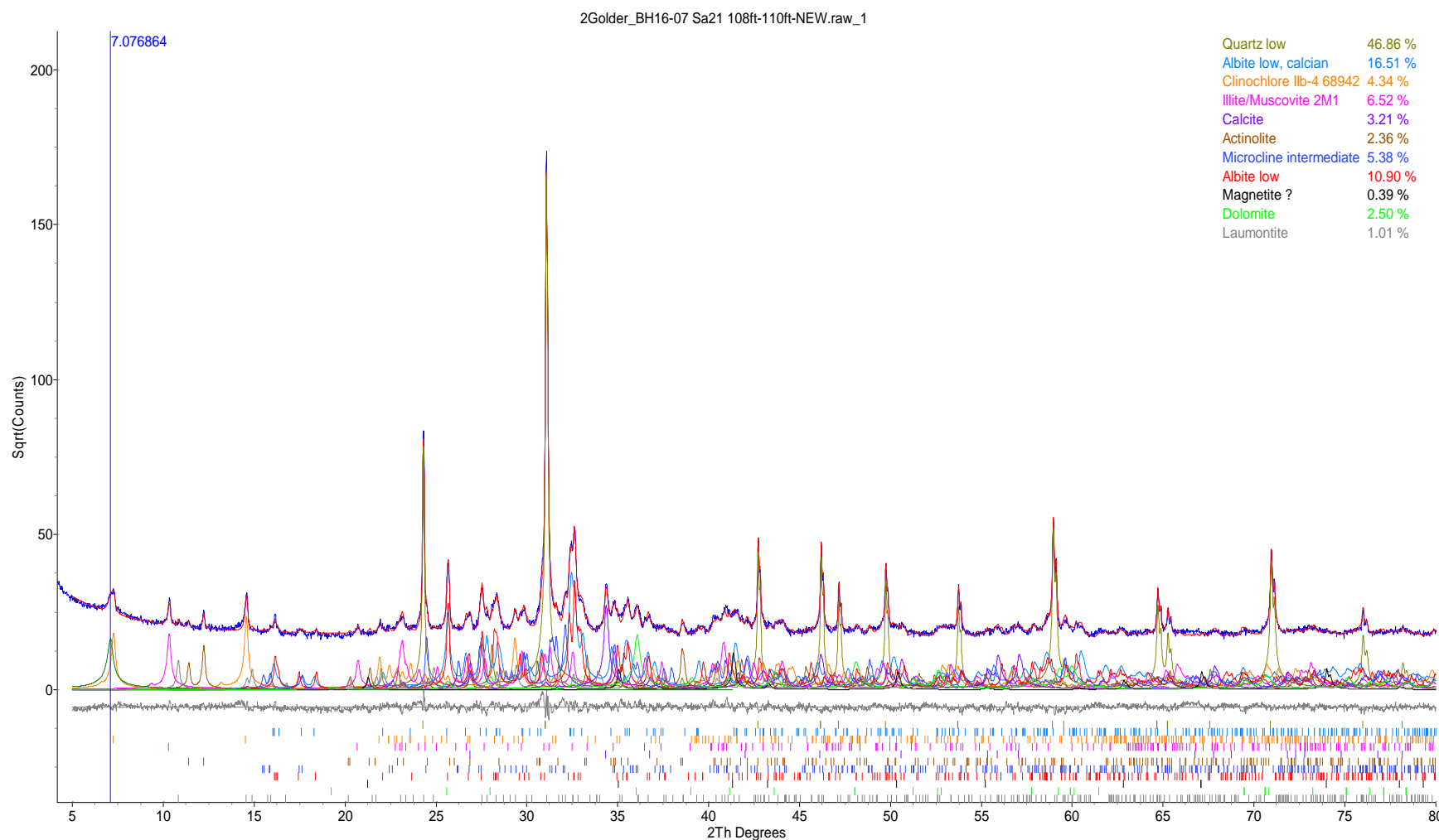
Figure 2. Rietveld refinement plot of sample Golder Associates BH16-07 Sa21 108'-110' (blue line - observed intensity at each step; red line - calculated pattern; solid grey line below – difference between observed and calculated intensities; vertical bars - positions of all Bragg reflections). Coloured lines are individual diffraction patterns of all phases.
