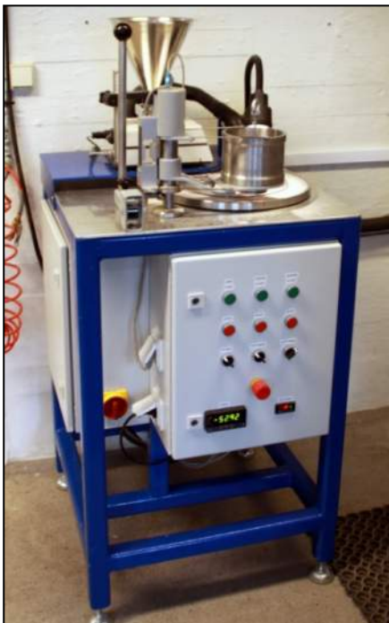
Figure 3. Photos of test equipment used to determine soil abrasivity by the Soil Abrasion Test (SAT™).
