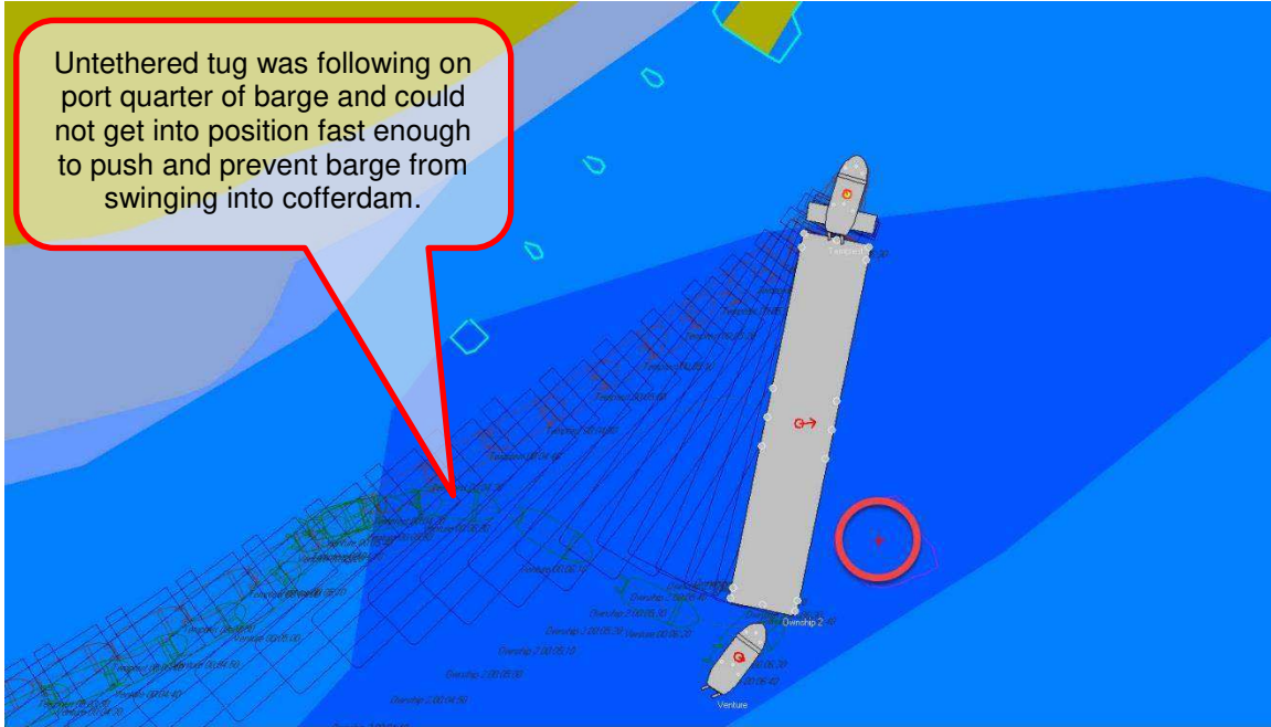
Figure 22: Run 14 Track Plot – Ebb Tide Arrival and Loss of Barge Control
