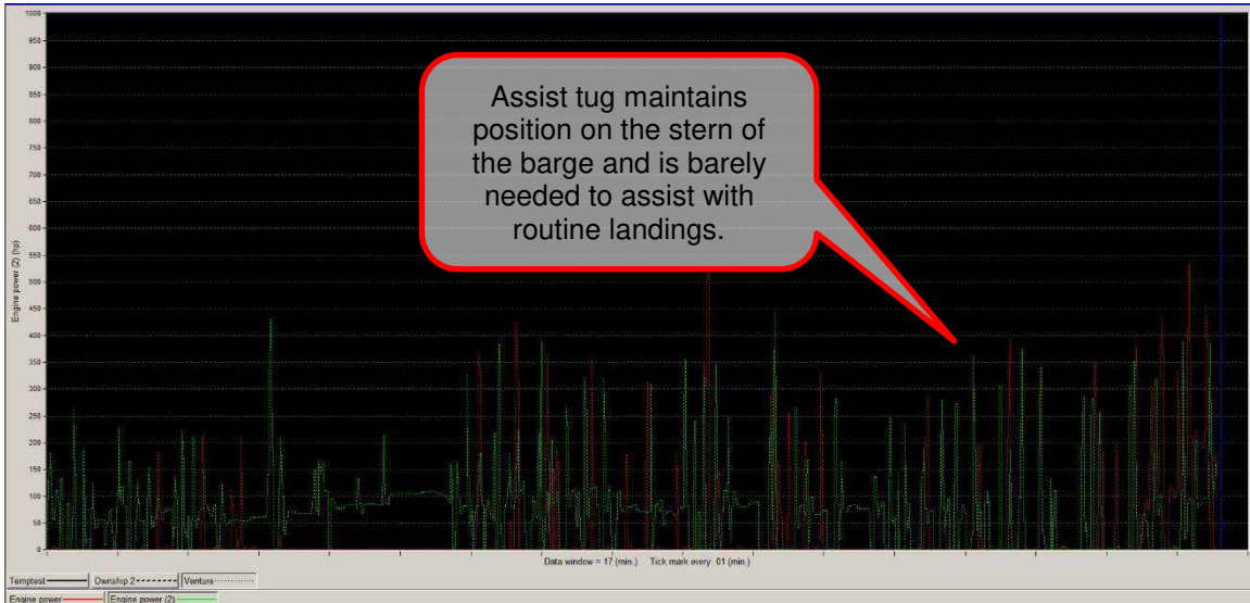
Figure 20: Assist Tug Engine Power Graph – Simulation Run 4
