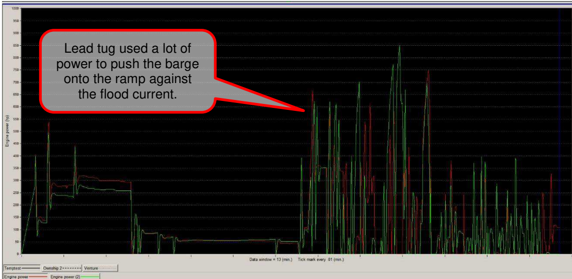
Figure 10: Lead Tug Engine Power Graph – Simulation Run 1
