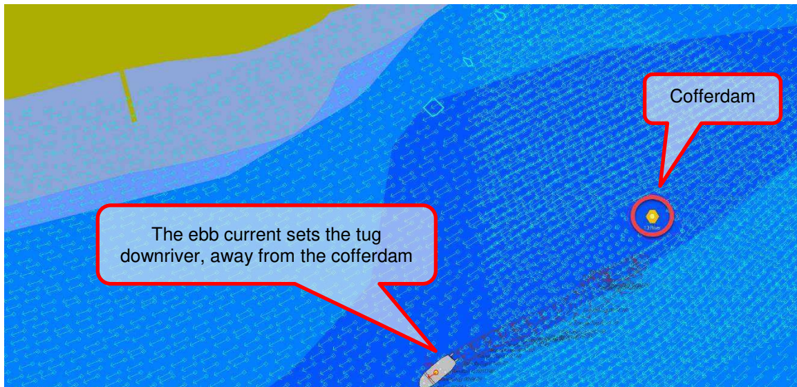
Figure 7: Current Drift Effects – Ebb Tidal Stream (Falling Tide) – Standby Tug
