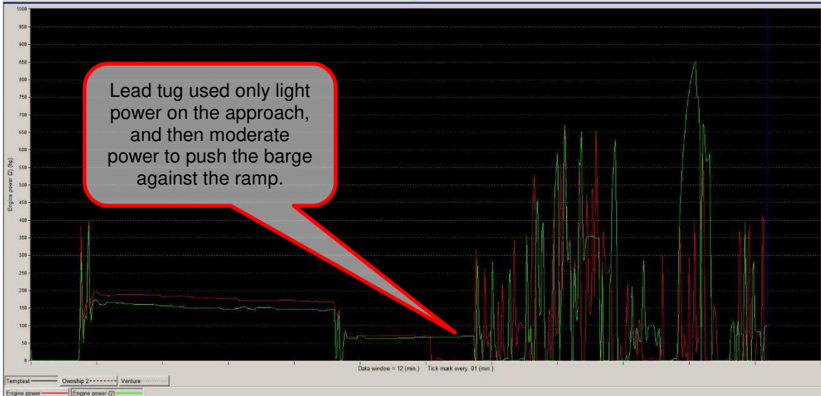
Figure 14: Assist Tug Engine Power Graph – Simulation Run 13
