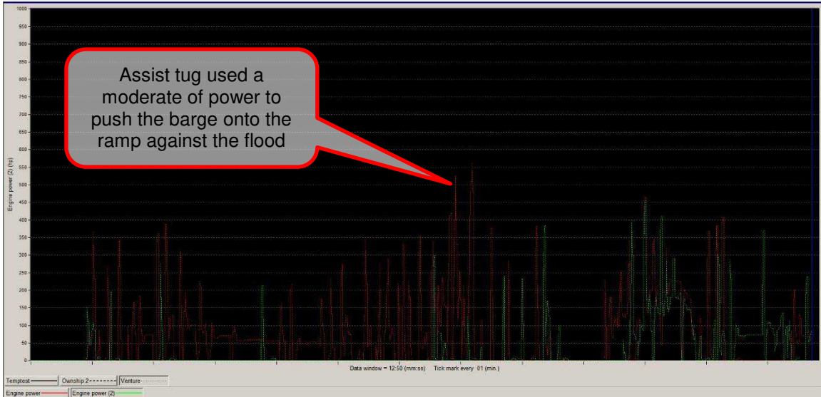
Figure 11: Assist Tug Engine Power Graph – Simulation Run 1
