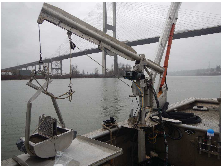
Photo 1: The Van Veen Sampler and Boom Used for the Sediment Collection Program
