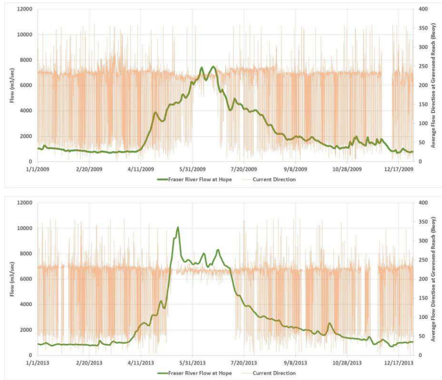
Figure 3-8. 2009 and 2013 Time Histories of Fraser River Flow at Hope and Current Direction at Gravesend Reach Buoy
