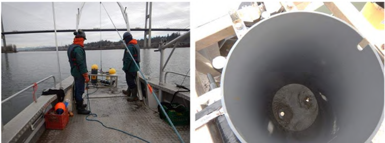
Figure 4: Frame redeployment on 14 February 2017 (Left) and Sand accumulation inside the EdgeTech rope canister (Right).
