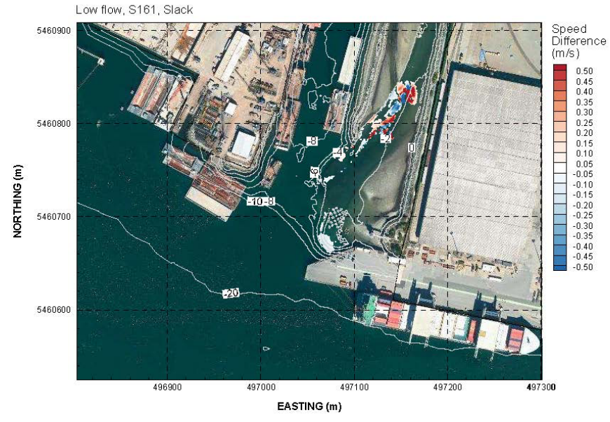
Figure B1 Velocity difference between the existing conditions and proposed design the offset footprint during low Lynn Creek discharge
