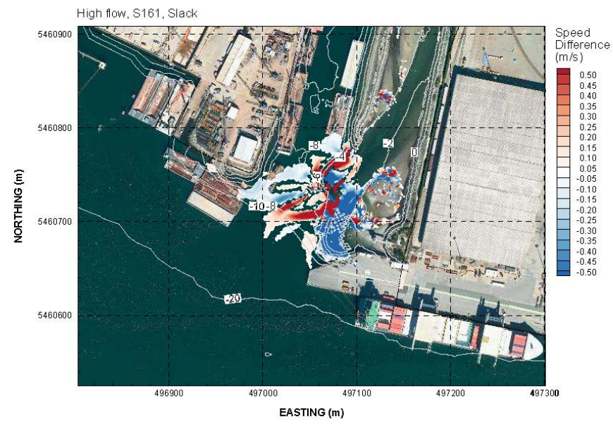
Figure B2 Velocity difference between the existing conditions and proposed design the offset footprint during high Lynn Creek discharge
